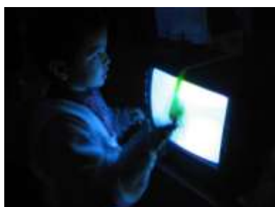
In a dark room, a young boy views the effects of a magnet on a television.
